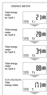
**Note:** the information **T23** on the display indicates that the corresponding phase (1,2,3) is under voltage.
